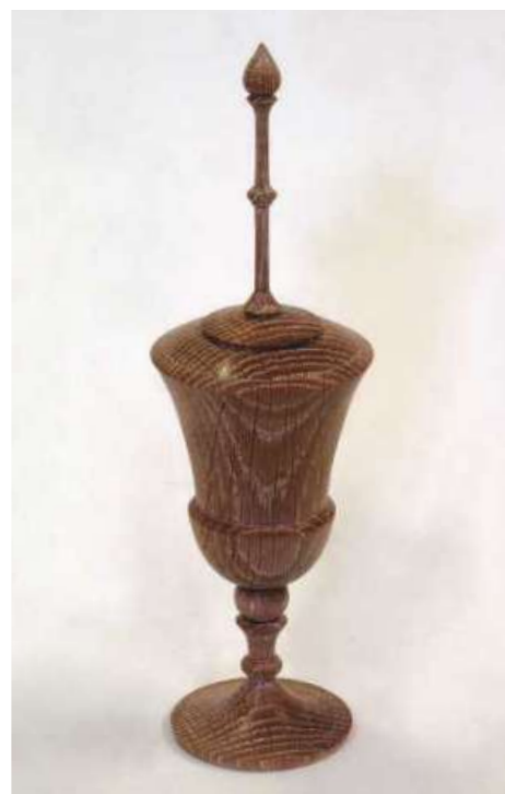
▲ Pic.35 The work is a little delicate for mounting on the lathe and cleaning up the underside of the base so Les mounted a sanding arbor in the pillar drill and progressed through the grits from 120 to 400
